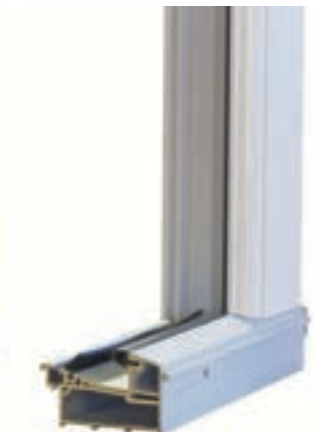
Stormguard Plus Rebated Threshold Distance from bottom of door leaf to bottom of threshold - 20mm . Available in Silver only. (Not wheelchair accessible)
